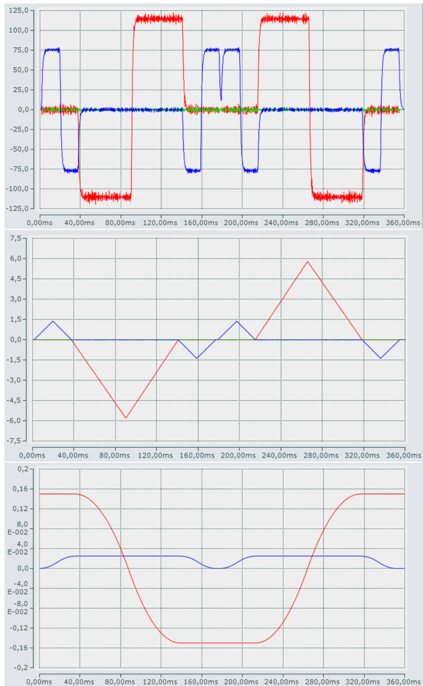
Figure 4.2: Graphs showing the Cartesian acceleration, velocity and position of the test cycle in millimetres. X: red, Y: green, Z: blue.
